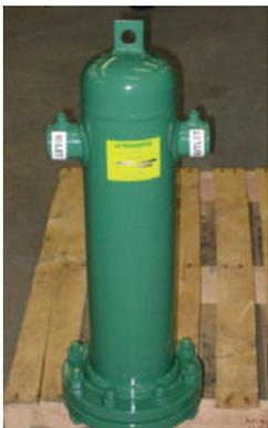
The Lectrodryer type SF and type F filters provide high efficiency filtration with ten sizes available in each type for flows to 8400 SCFM, larger sizes available on application. Both types have a high level filter efficiency of 99.985% retention (0.015 DOP penetration) for filtration to a 0.3 micron particle size and smaller.
