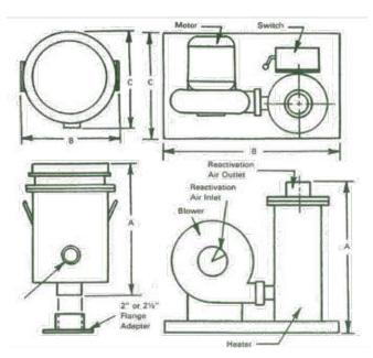
Simplification has been emphasized in the design of the Lectrobreather. A flanged adapter is provided for the storage tank vent to receive the Lectrobreather, which then seals itself on a soft gasket by virtue of its own weight. Removal for reactivation requires merely lifting and placing on a similar adapter on the reactivator. Fool-proof operation is assured with a minimum of maintenance.
