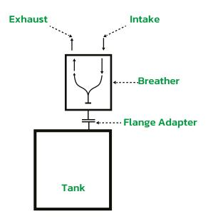
It is suggested that the Breather be mounted directly on tank when material is non-corrosive.
