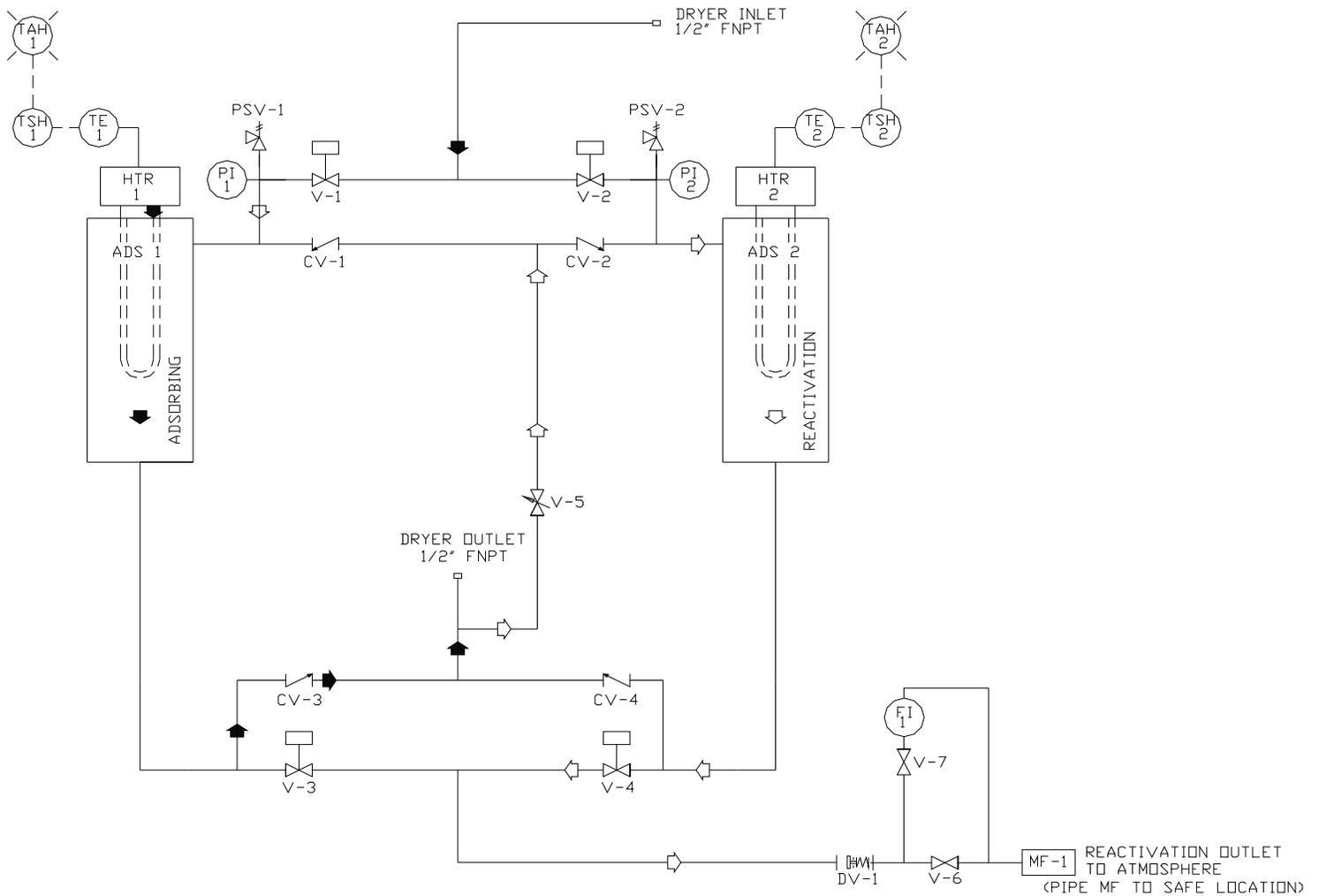
The wet gas enters the HPB Lectrodryer at the adsorption inlet. Flow is directed to the left adsorbing tower, adsorber 1, and is dried passing through the desiccant bed. The dryer gas exits through the bottom dryer outlet.
