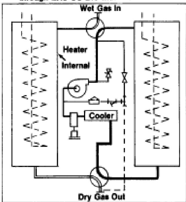
Typical flow diagram for models GAS-CC-350 through GAS-CC-3500 with external heater.
